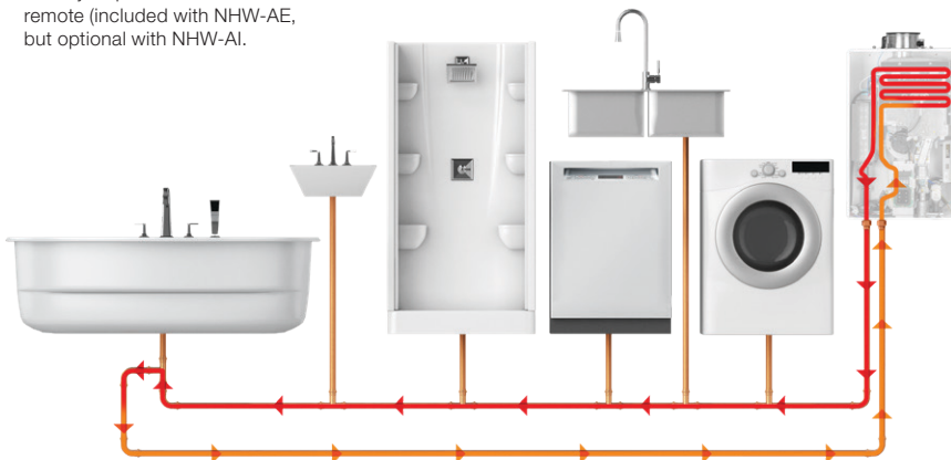
External recirculation with dedicated recirc loop
