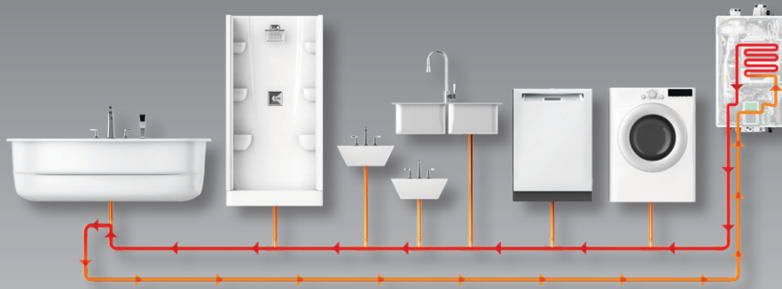
ComfortFlow® built-in recirculation system available on NPE-A2 and NHW-A models
