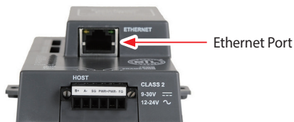
Figure 14: Ethernet Port Location
