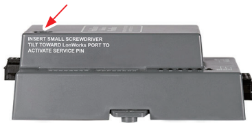
Figure 22: LonWorks Service Pin Location
