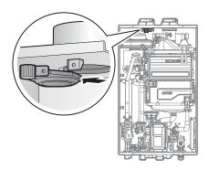
6. Remove the filter from the plastic assembly and clean it with a toothbrush and clean running water.
