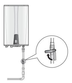
5. Open all hot water faucets completely. The water that remains in the plumbing lines will drain out.
