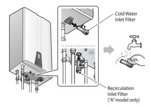
3. Reinsert and tighten the filters.
